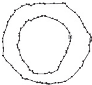
Even such a ragged edge doesn't need this many points! More points means more data that has to be processed by the printer.
